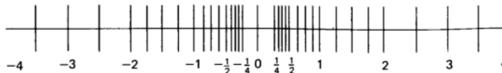
Fig. 2.1. The floating-point number system for \beta = 2 , t = 3 , L = -1 , U = 2 .
