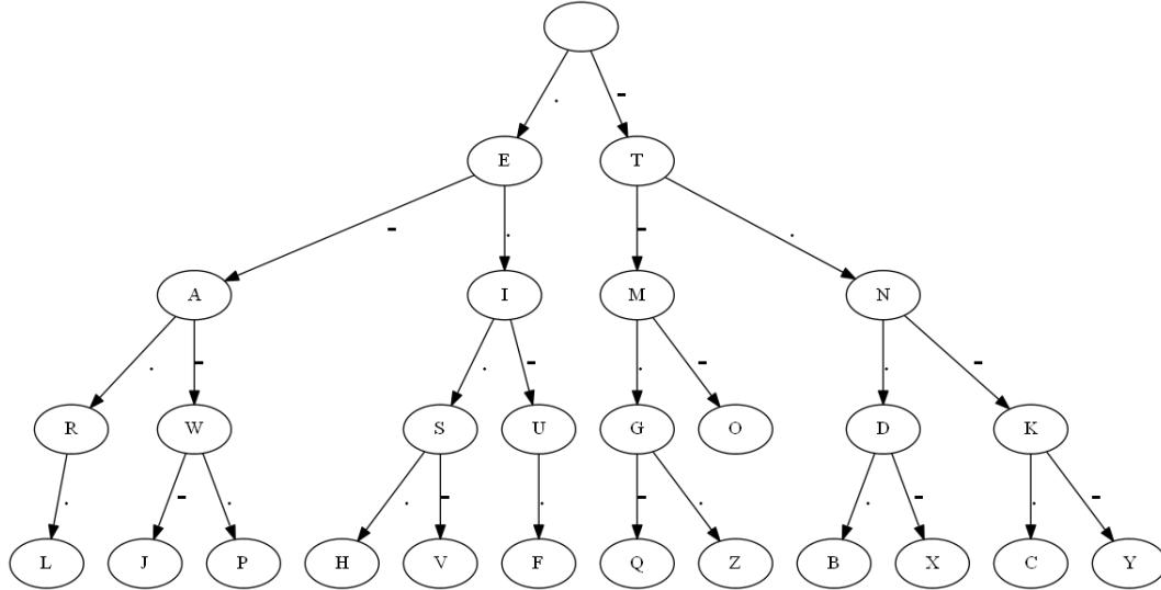
This yields a simple method of decoding in real time as each “dot” and “dash” is received. We simply trace the path in the tree until we find the appropriate letter.
