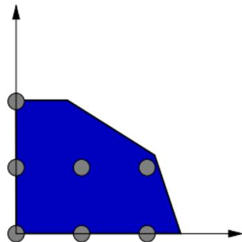
$$\begin{aligned} S &= \{(x_1, x_2) \in \mathbb{Z}_+^2 : 6x_1 + x_2 \leq 15, \\ &\quad 5x_1 + 8x_2 \leq 20, x_2 \leq 2\} \\ &= \{(0, 0), (0, 1), (0, 2), (1, 0), \\ &\quad (1, 1), (1, 2), (2, 0)\} \end{aligned}$$
