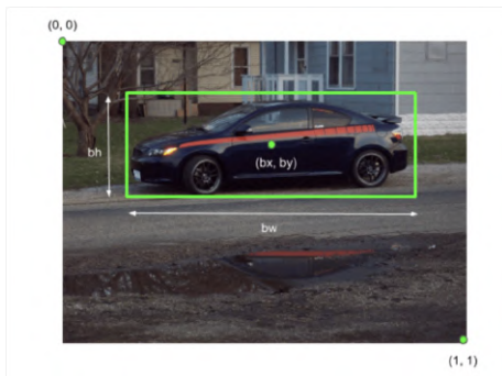
Figure: Bounding box representation used for object localization
