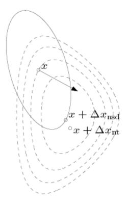
dashed lines are contour lines of f; ellipse is  $\{x+v\mid v^T\nabla^2f(x)v=1\}$  arrow shows  $-\nabla f(x)$
