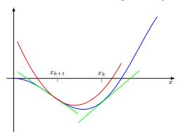
Secant equation  $H_k y_k = s_k$  to match gradient of f at  $w_k$ , where
